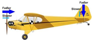
surfaces are. If you slow way down to just above stall speed, the control surfaces have only marginal effect and aren't very effective is preventing a ground loop. The slower you are going, the less effective the elevator is in keeping your tail down.
